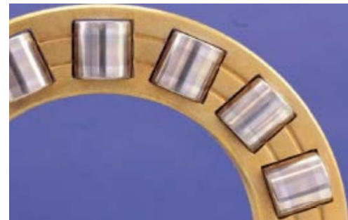
Low visible bearing roller & cage wear (FAG FE-8)
