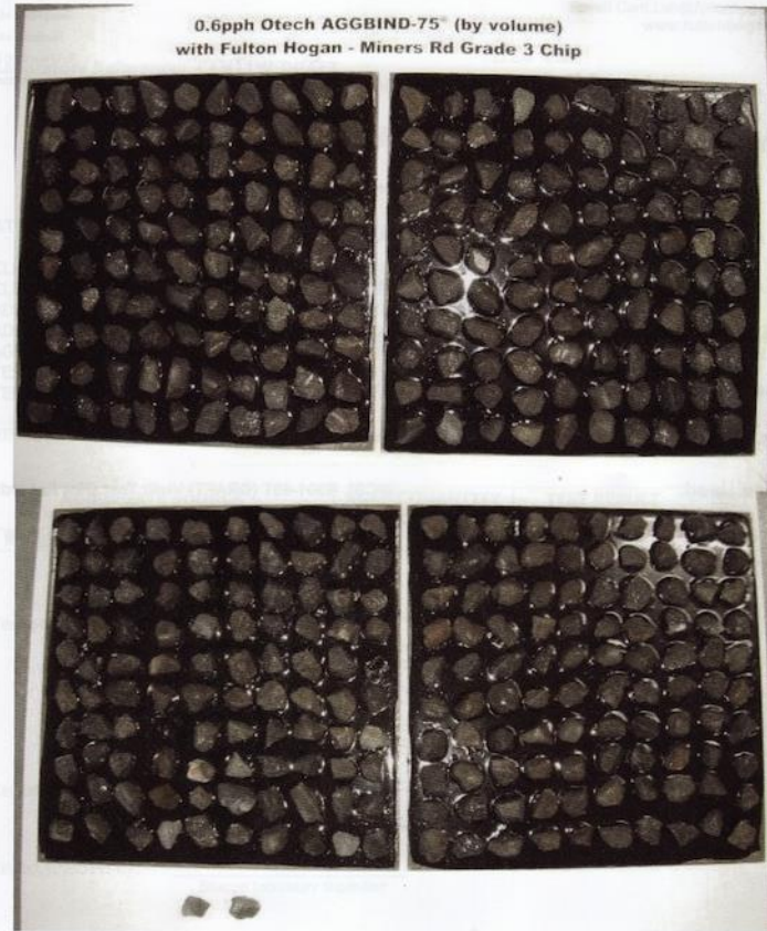
Figure 1. Photograph showing test plates with 180/200 bitumen and 0.6pph Otech AGGBIND-75 ® (by volume) after test was performed. Fulton Hogan – Miners Rd grade 3 chip that was dislodged is arranged below the plates.
