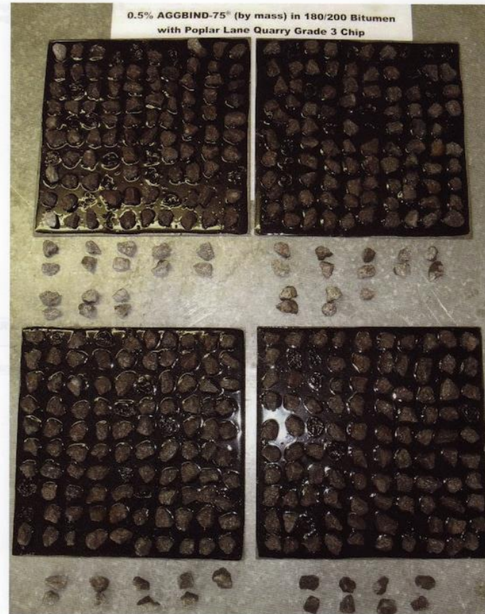
Figure 1. Photograph showing test plates with 180/200 bitumen and 0.5% Otech AGGBIND-75 ® (by mass) after test was performed. Poplar Lane Quarry grade 3 chip that was dislodged is arranged below the plates.
